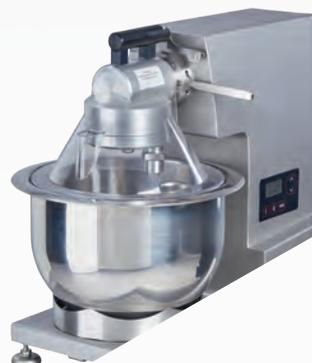
**Planetary stirring, beating and kneading unit 15 l**
