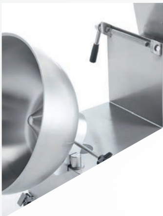
Bowl may be tilted to the front for easy discharge
