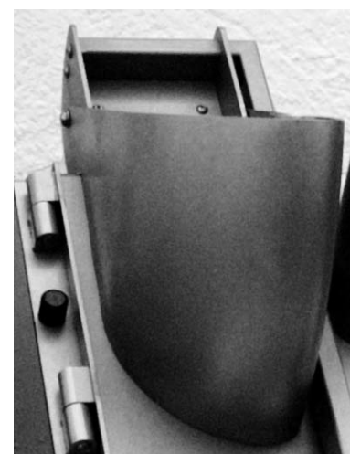
Großzügiger Einfüllschacht für sperrige Rohwaren. Pusher to make full use of the material during cutting process.
